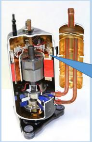
Copper wire and tube are used as main parts in the compressor.
